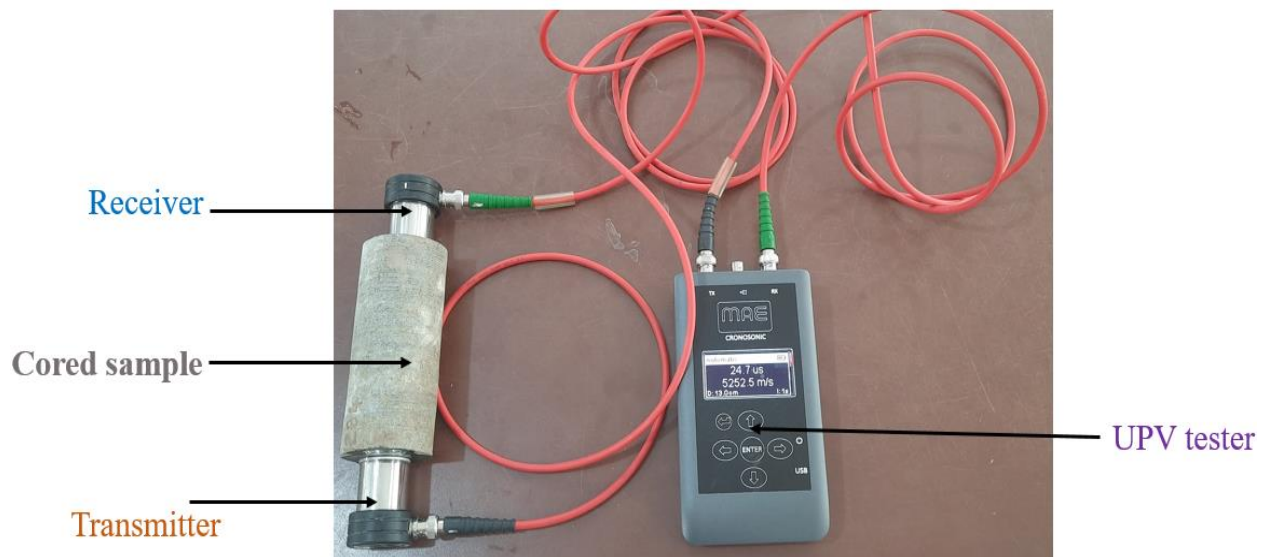
Figure 2: Laboratory determination of P-wave velocity
